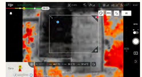
Image: A thermal camera image comparing surface roof temperatures on a home in Burkina Faso (see next page ). The cool roof side is 30.1°C; the unmodified side is 44.1°C.
